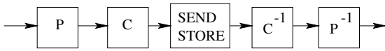
Figure 1: The preprocessing takes place before the actual compression and is reversed after decompression.
