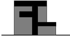
Figure 1: Illustration of Fitness Functions. The structure itself is black, and the grey region is considered “shaded”. In the first fitness function, which measures the “coverage” by summing maximum column heights, both the black and grey areas of the figure are counted. The second fitness function, “shading”, only measures the grey area.
