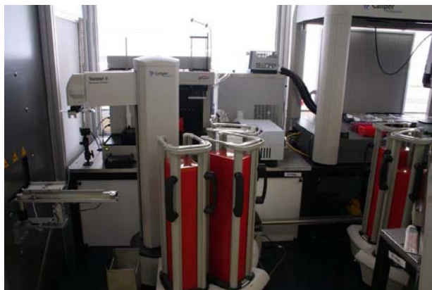
Figure 1: The hardware system of our Robot Scientist. Visible here are one of the robot arms (twisters). The automated freezer library in which yeast strains are stored is on the left and the chemical dispenser is on the right. Several other components, including plate readers and incubators, are not shown.
