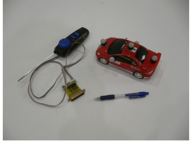
Figure 1: The toy car and its remote, note the reflecting markers.
