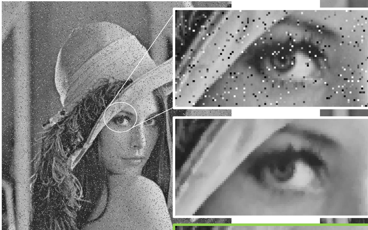
corrupted image (10% pixels, impulse noise)
